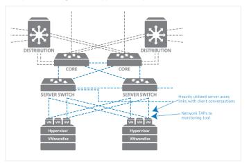
Figure 3. Instrumenting the application server access layer to avoid traffic congestion
