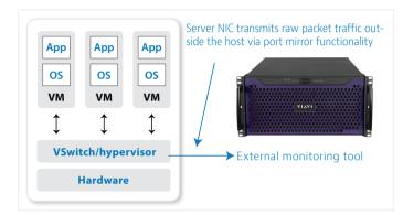
Figure 2. The outside virtual monitoring model: all analysis is performed externally
