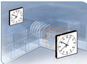
**PATENTED FREQUENCY-HOPPING TECHNOLOGY** - This patented technology allows each clock to frequency hop the transmission to all of the surrounding clocks, enabling it to receive the correct time, even if there is interference on any of the frequencies.
