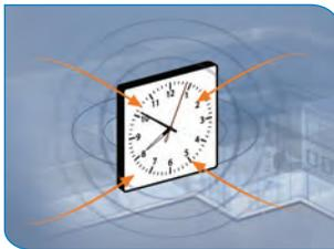
**RECEIVES SIGNAL FROM MULTIPLE PATHS** - Since each clock has a repeater built-in, the wireless signal can be received from any clock in the signal's radius.
