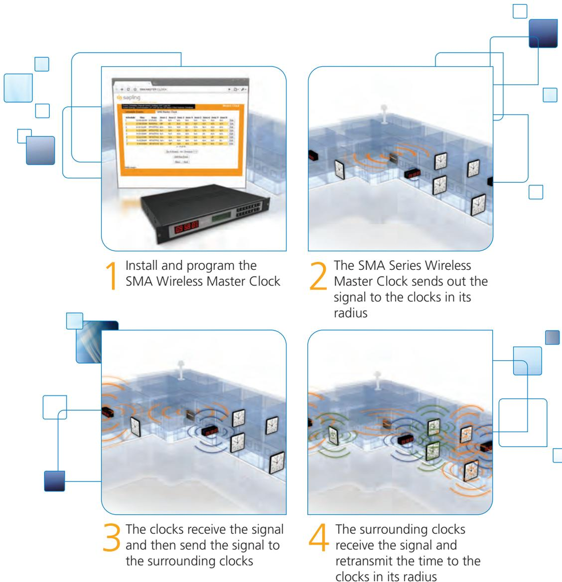
**Sapling's Wireless Clock System** is the embodiment of innovation and reliability. Eliminating wiring throughout an entire facility can save you thousands of dollars on installation and also allows for retrofitting of an existing installation. While most wireless systems are limited to the range of the transmitter, Sapling's is not.
