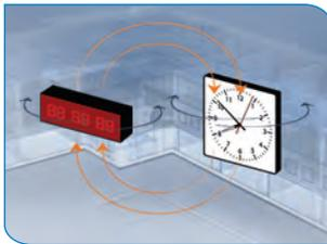
**EACH CLOCK HAS A REPEATER BUILT-IN** - Since each clock has a repeater built right into each unit, there is no need for high power transmitters and repeaters. Each clock receives the wireless signal and sends out the time to its neighboring clock, making Sapling's system unique and extremely accurate.
