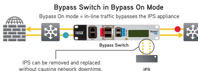
By logging into the device from anywhere on the network, operators can monitor traffic and device status, and configure and control the device. One aspect of device control is the ability to force the bypass switch into Bypass On mode, taking the IPS offline. This capability can be handy for easily removing the IPS from service without requiring a technician to be physically on site with the IPS, saving time and travel costs.
