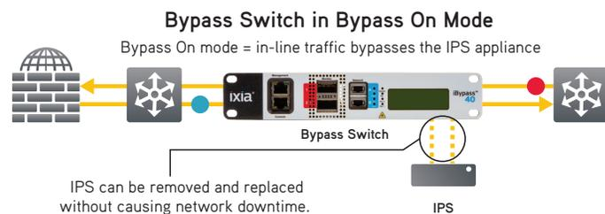
By logging into the device from anywhere on the network, operators can monitor traffic and device status, and configure and control the device. One aspect of device control is the ability to force the bypass switch into Bypass On mode, taking the IPS offline. This capability can be handy for easily removing the IPS from service without requiring a technician to be physically on site with the IPS, saving time and travel costs.
