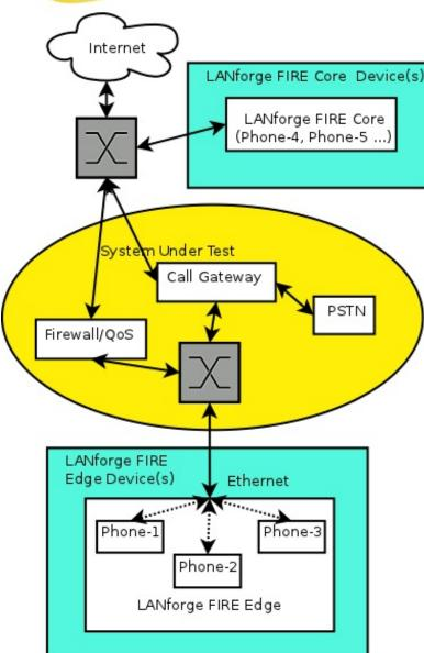
LANforge FIRE supports multiple Ethernet and Virtual interfaces. To the System Under Test, it appears as if each interface is a separate PC or network appliance generating independent stateful traffic streams.
