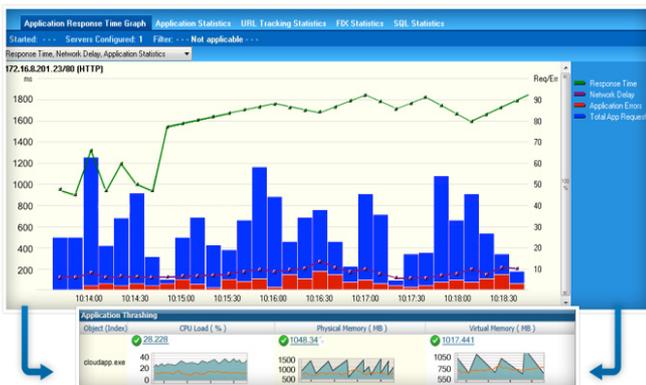
For example, poor response time of an application hosted on a virtualized server may have nothing to do with the service or the network, but may instead be tied to excessively high CPU utilization. Without this monitoring perspective, troubleshooting will be more difficult and time consuming.
