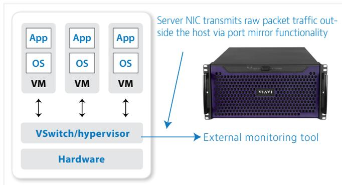
Figure 2. The outside virtual monitoring model: all analysis is performed externally
