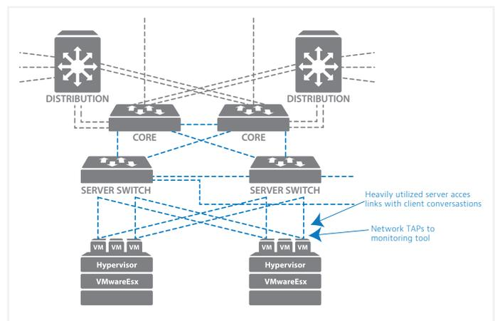
Figure 3. Instrumenting the application server access layer to avoid traffic congestion
