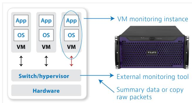
Figure 1. The inside virtual monitoring model: virtualized server monitoring using a VM monitor instance
