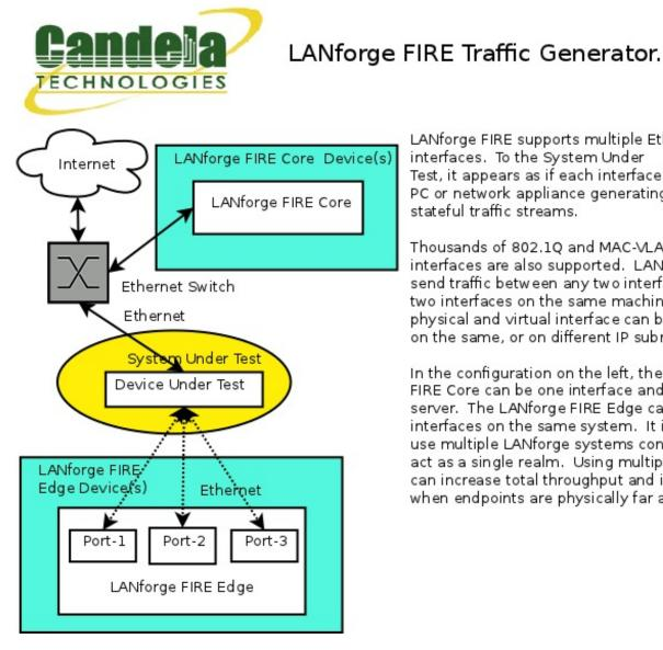
LANforge FIRE supports multiple Ethernet interfaces. To the System Under Test, it appears as if each interface is a separate PC or network appliance generating independent stateful traffic streams.
